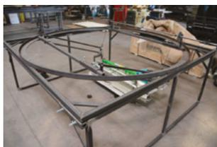
This frame has a revolutionary design: it can be used for a SUPERCUT machine with a cutting width of either 1200 mm or 1600 mm! It measures 2 m x 2 m.
